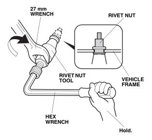
Remove the rivet nut tool from the rivet nut by turning the hex wrench counterclockwise.  Position left bracket A onto the vehicle frame in the area shown, and loosely install it using two flange bolts. Do not tighten the flange bolts at this time. Make sure the flange bolts are installed into the correct locations.
