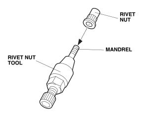
Insert the rivet nut into the hole in the vehicle frame and install the hex wrench on the rivet nut tool.
