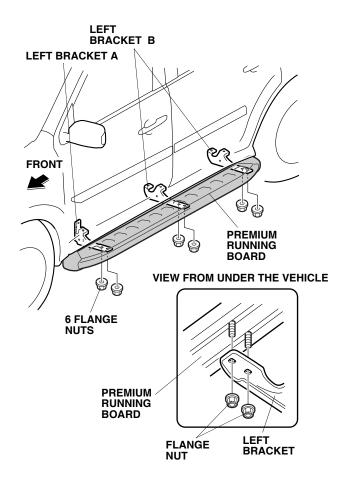
6. Center the premium running board on the left side of the vehicle, and tighten the six flange nuts loosely installed in step 5. Torque the flange nuts to 27 N·m (19 lbf·ft).
