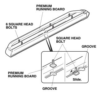
Position the premium running board onto the left brackets, align the square head bolts with the holes in the brackets and loosely install the six flange nuts.
